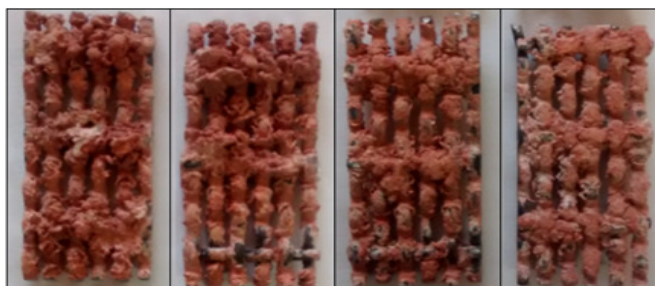
Figure 8. Metallic screen samples encrusted with mud crust.
